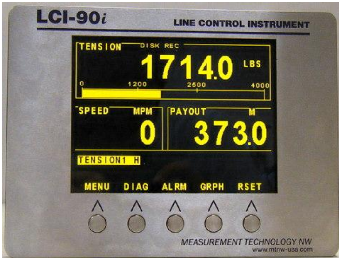
Figure 1.1 – LCI-90i Front Panel
