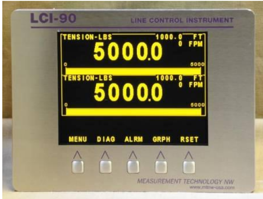
Figure 5.7 – LCI-90i Dual Winch Mode
