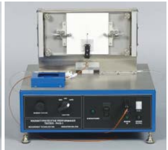
RPP Device with sample tray in place (left) and with calorimeter sensor in place (right)
