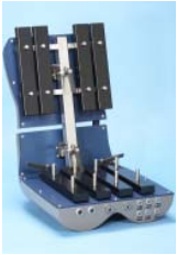
All-new STAN manikin for seat testing.
